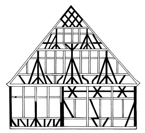
Gable of the water castle of Balingen The beams that are traced in black clearly indicate the Runes, which in most cases were not essential elements of the structure.
